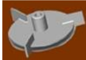
Rushton turbine with three blades.
